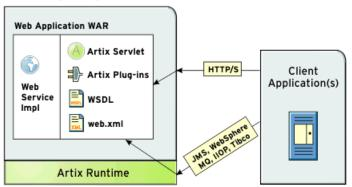
Figure 7: Exposing Artix Web Service from a Servlet Container
