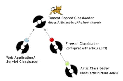
Figure 8: Classloader Configuration
