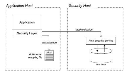
Figure 25: Locally Deployed Action-Role Mapping ACL File
