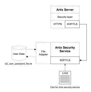
Figure 3: An IIOP/TLS Connection in the HelloWorld Example
