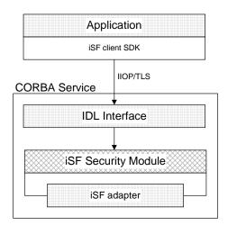
Figure 34: iSF Server Module Deployed as a CORBA Service
