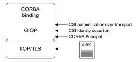
Figure 7: Protocol Layers in a CORBA Binding
