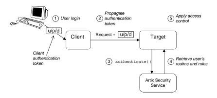
Figure 13: Two-Tier CORBA System Using CSI Credentials
