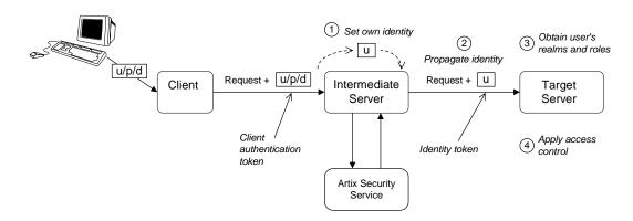
Figure 14: Three-Tier CORBA System Using CSIv2
