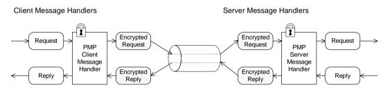
On the client side, the outgoing request passes along the chain of handlers until it reaches the PMP SOAP message handler, which encrypts the message's SOAP body.
