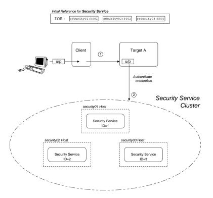
In this scenario, it is assumed that both the client and the target application are configured to perform *random load balancing* over the security services in the cluster (see "Client Load Balancing" on page 231 for details). Each of the security services in the cluster are configured for failover.
