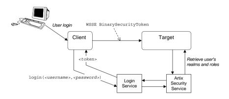
Prior to contacting the target server for the first time, the client Bus sends the username, <username>, and password, <password>, to the login server, getting an SSO token, <token>, in return. The client Bus then includes an IONA-proprietary SOAP header (extension of WSS BinarySecurityToken) in the next request to the target server. The target server's Bus contacts the Artix security service to validate the SSO token passed in the WSS Binary SecurityToken.
