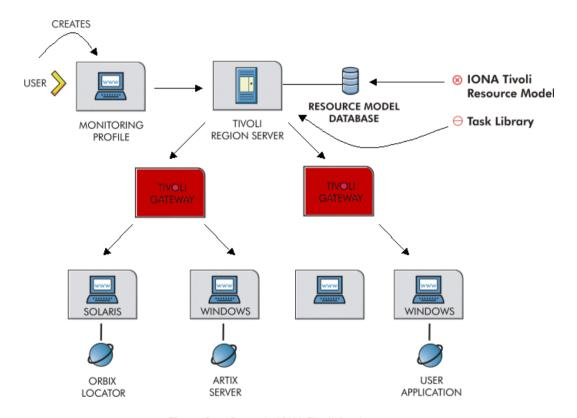
Figure 2: Example IONA Tivoli Deployment
