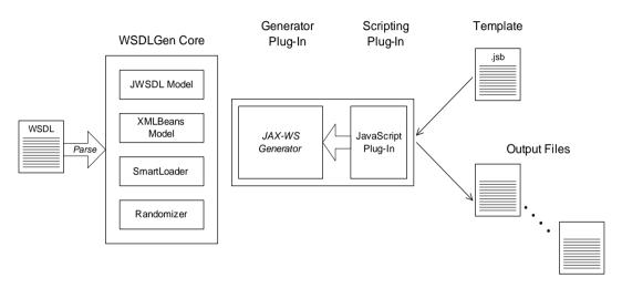
Figure 1: WSDLGen Code Generator Architecture
