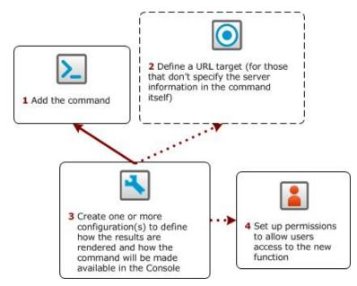
A basic integration requires a command and a configuration. You can create families of related commands that use different parameters for different contexts by creating additional configurations. A target is required if the service is a web service (web URL).
