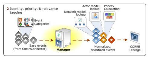
The SmartConnector sends the aggregated and filtered events to the Manager, where they are evaluated and tagged with network and actor modeling information, and priority levels, then stored in CORR-Engine storage.
