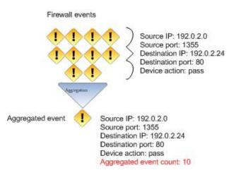
If the 30-second time frame expires and the connector has received only two matching events, the connector will create a single aggregated event with an aggregated event count of two. If 900 matching events come in during the 30 seconds, the connector would create 90 aggregated events, each with an aggregated event count of 10.
