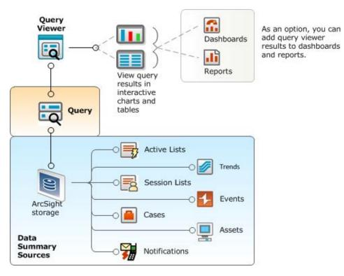
Query viewers combine the SQL querying ability of trends and reports with the drill-down capabilities of active channels in a single resource. The flexibility of SQL queries with access to drill-down details enables you to track how a situation is developing in real time. Querying the focused data set of a trend table is more performance friendly than creating low-level active channels.
