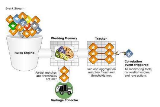
The rules engine evaluates the event stream, holds matches in working memory, and processes join and aggregation conditions in the tracker. If all conditions are met within the time thresholds, a correlation event is triggered.
