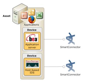
**Asset** is the term ESM uses to describe a network node with a unique identifier (IP or MAC address, host name, zone, or external ID) in the ESM network model. This example shows one asset that hosts two devices and a series of applications. Details about the asset will appear in the Device fields of the events reported by the BEA application server and the Cisco HIDS.
