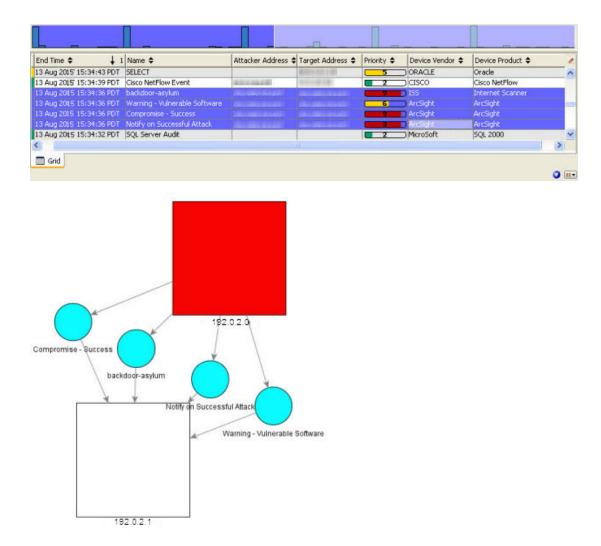
This graph shows the events that indicate a successful backdoor asylum attack on an ISS web server. In the ArcSight Console, you can double-click any node to investigate its origin.
