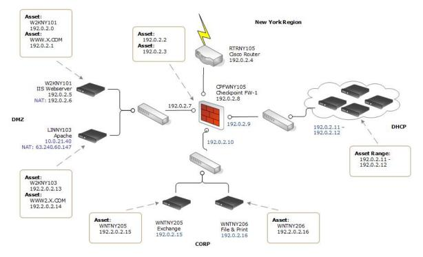
The diagram below shows assets and asset ranges in the example network.
