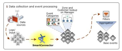
A data source on a network node generates events, which are collected by an ArcSight SmartConnector. The connector normalizes the data into the ESM schema, then tags it with event categories and looks up zone and customer attributes from the ESM network model. You can also configure the SmartConnector to filter and aggregate events to reduce the volume of the event stream.
