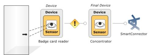
A sensor is the component of a device that actually detects the activity. Devices can report to a SmartConnector through a chain of multiple devices.
