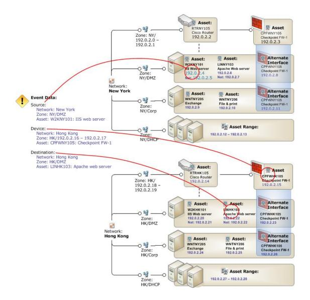
When an event comes into the system, the Manager uses the network model to identify the assets involved in the event. In this example, the endpoints involved in the event are circled in red.
