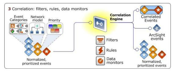
Events that have been tagged with event categories, priority evaluations, and network model information are then processed by the correlation engine, where filters, rules, and data monitors connect the dots, find the events of interest, and can initiate immediate response.
