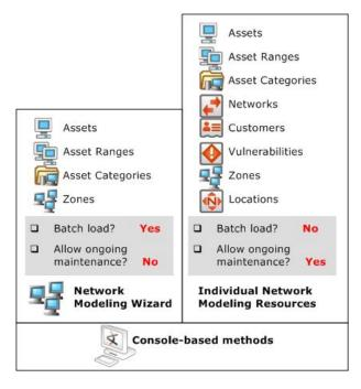
All the individual tools for modeling the network are available in the Console. The Network Modeling Wizard provides a quick way to add basic assets to your Network Model at ESM setup time.
