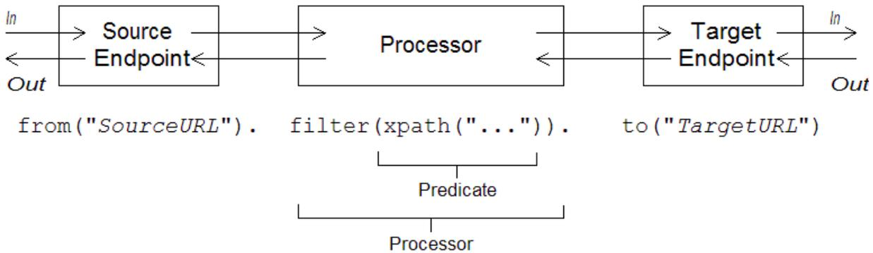
A local rule always starts with a `from("EndpointURL")` method, which specifies the source of messages for the routing rule. You can then add an arbitrarily long chain of processors to the rule (for example, `filter()`), finishing off the rule with a `to("EndpointURL")` method, which specifies the target for the messages that pass through the rule. It is not always necessary to end a rule with `to()`, however. There are alternative ways of specifying the message target in a rule.
