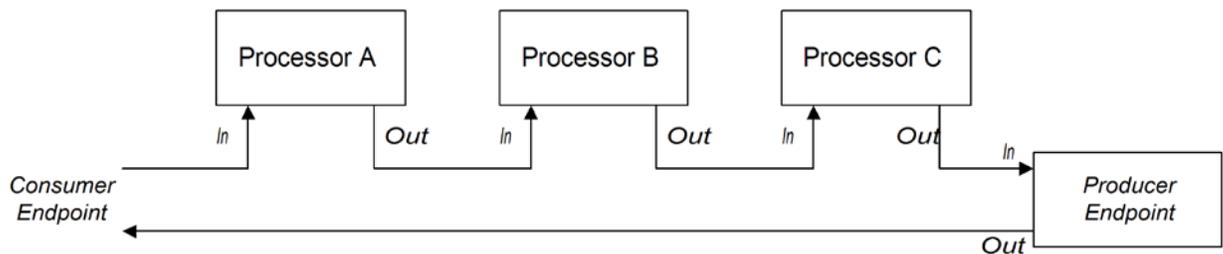
Note that in order to support the *InOut* exchange pattern, it is *essential* that the last node in the route (whether it is a producer endpoint or some other kind of processor) creates an *Out* message. Otherwise, any client that connects to the consumer endpoint would hang, waiting indefinitely for a reply message. In particular, you should be aware that not all producer endpoints create *Out* messages.
