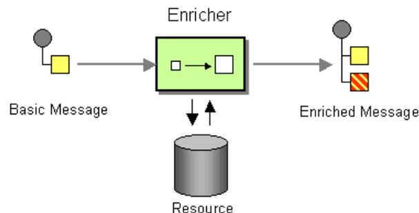
The key difference between the content enricher approach and the segmented route approach is that the content enricher is based on a radically different event model. In the segmented route
