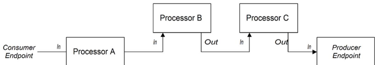
Java Router employs the pipeline pattern by default. Hence, you do not need to use any special syntax to create a pipeline in your routes. For example, the following route pulls messages from a `userdataQueue` queue, pipes the message through a Velocity template (to produce a customer address in text format), and then sends the resulting text address to the queue, `envelopeAddressQueue`:
