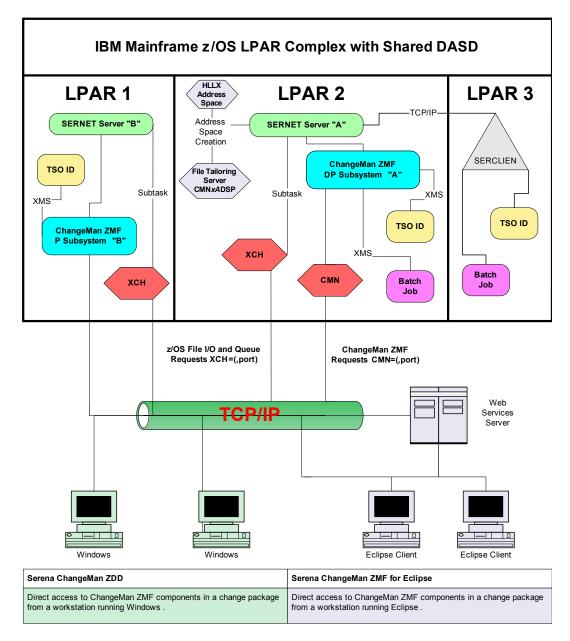
The diagram shows two Sernet instances on separate LPARs, each managing a ChangeMan ZMF instance. Users access these ChangeMan ZMF instances from the Web, from workstations in the distributed environment, and from TSO sessions in the z/OS environment. The TSO user in the last LPAR is using the Load Balancing Option of ChangeMan ZMF to work from a mainframe environment where there is no Sernet or ChangeMan ZMF instance.
