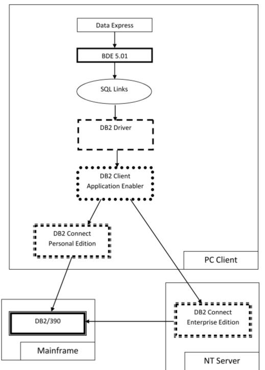
BDE is inserted on another layer, the Borland SQL Links layer, which is installed together with BDE.
