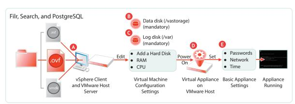
Figure 2-7 A Small Deployment of Filr on VMware
