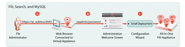
Figure 2-9 Configuring an All-in-One Filr Appliance
