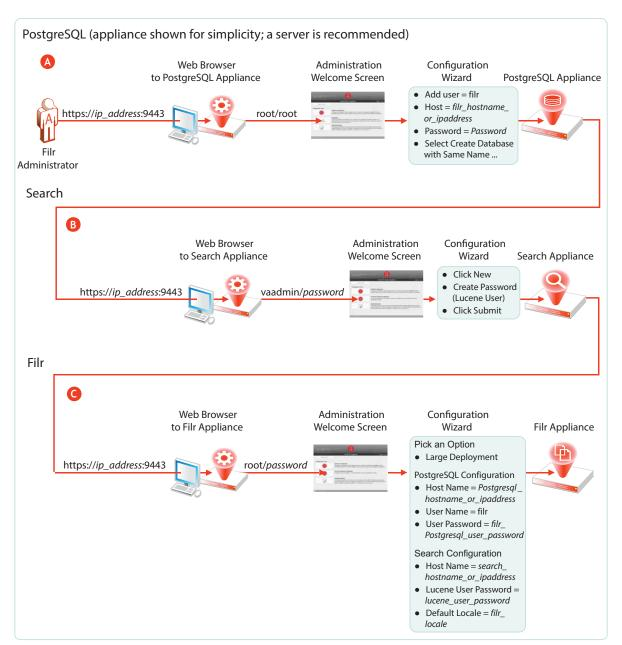
Figure 2-10 Configuring Separate Appliances
