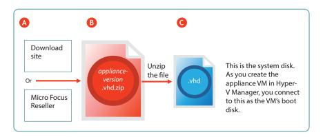
Figure 2-1 Downloading and Preparing OpenText Appliances for Hyper-V
