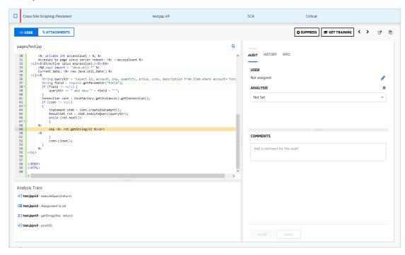
**Note:** This screen capture shows the details for an issue uncovered during a Fortify Static Code Analyzer scan. For information about viewing Fortify WebInspect results, see "Viewing Fortify WebInspect Scan Results in Fortify Software Security Center" on page 319.
