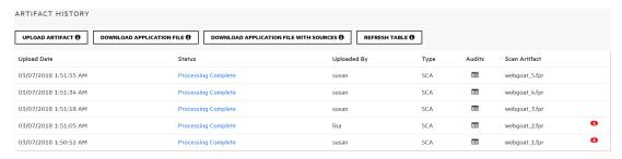
2. To open the SCAN WARNINGS or SCAN ERRORS window and view detailed information about the errors encountered, click the number in the red circle.
