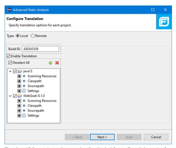
The selected Eclipse projects to be scanned are listed in the left pane. To exclude a project from the advanced analysis, clear the check box for the project.
