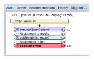
For dataflow issues, the trace starts with the first function to call the taint source, then traces the calls to the source (blue node) and ends the trace at the sink (red node). In the diagram, the source (src) and sink nodes are also labeled. A red X on a vertical axis indicates that the called function finished executing.
