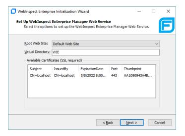
If you have configured HTTPS bindings for the root web site in IIS, only those bindings will be listed in the Available Certificates. You will not be able to create a new binding for a web site in the Fortify WebInspect Enterprise Initialization Wizard. You can create a new binding only in IIS. The following table describes your options, based on your IIS settings.
