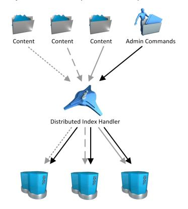
The DIH distributes the index data that it receives (represented by gray arrows in the diagram above) evenly across the connected IDOL Servers. For example, if the DIH connects to four IDOL servers, it indexes approximately one quarter of the data into each IDOL server. It does not split up sections of individual documents.
