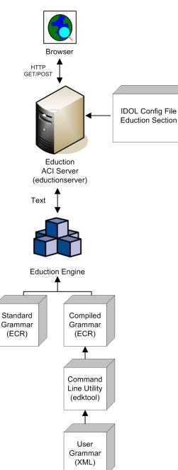
Figure 3: Extraction using the Eduction ACI Server
