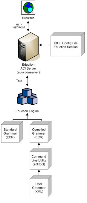
Figure 3: Extraction using the Eduction ACI Server
