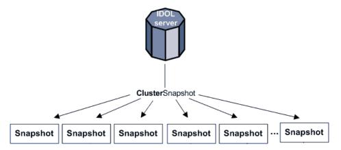
The ClusterSnapshot action allows you to take a snapshot of the data stored in the HPE IDOL Server data index. By default this includes data for the HPE IDOL Server databases News and Archive. A snapshot represents the content of the data index at a particular time, and enables you to generate cluster information and spectrographs at a later point, even if the data index has changed. You can use a single snapshot to generate both cluster information and spectrograph data to save processing time.
