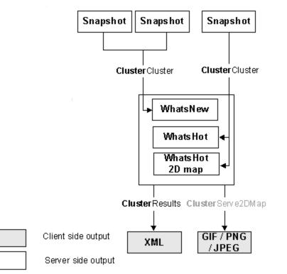
Clustering is a multistage hybrid algorithm. After the HPE IDOL Server Adaptive Probabilistic Concept Modelling (APCM) technology identifies similar documents, a hierarchical agglomerative clustering algorithm groups documents into conceptually similar areas. Dynamic binding and fixating produces the required clusters. The title is generated automatically by cross-correlating important concepts in a cluster with concepts in the titles of documents in that cluster.
