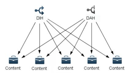
Depending on the size or requirements of the system, you can either use mirror mode for fault tolerance, or non-mirror mode for performance. You can also use chained DIH and DAH servers to allow for both.
