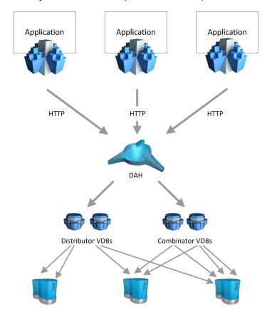
The DAH uses either combinator or distributor virtual databases (VDBs) to distribute the actions to one or more specific IDOL Server databases. The VDBs can map to one or more IDOL Server databases, or to other virtual databases that you set up for the DAH. The way a VDB forwards actions depends on its type.
