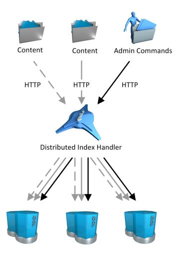
The DIH sends all the index data that it receives (represented by gray arrows in the diagram) to all the connected IDOL Servers. The IDOL Servers are exact copies of each other, and must all have the same configuration.
