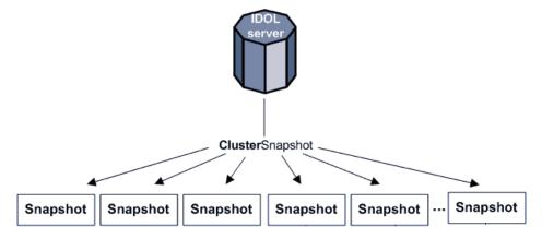
The ClusterSnapshot action allows you to take a snapshot of the data stored in the IDOL Content component data index. By default this includes data for the Content databases News and Archive. A snapshot represents the content of the data index at a particular time, and enables you to generate cluster information and spectrographs at a later point, even if the data index has changed. You can use a single snapshot to generate both cluster information and spectrograph data to save processing time.
