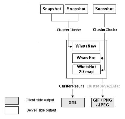
Clustering is a multistage hybrid algorithm. After the IDOL Adaptive Probabilistic Concept Modelling (APCM) technology identifies similar documents, a hierarchical agglomerative clustering algorithm groups documents into conceptually similar areas. Dynamic binding and fixating produces the required clusters. The title is generated automatically by cross-correlating important concepts in a cluster with concepts in the titles of documents in that cluster.
