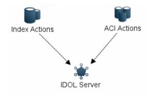
The unified setup uses the IDOL Proxy component. IDOL Proxy acts as a single point of contact for all your IDOL requests. It forwards all requests to the appropriate component. For example, it sends a
