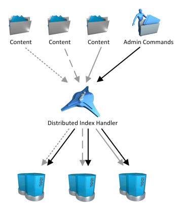
The DIH distributes the index data that it receives (represented by gray arrows in the diagram above) evenly across the connected IDOL Servers. For example, if the DIH connects to four IDOL servers, it indexes approximately one quarter of the data into each IDOL server. It does not split up sections of individual documents.
