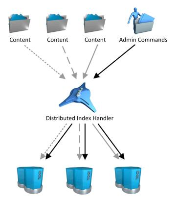
The DIH distributes the index data that it receives (represented by gray arrows in the diagram above) evenly across the connected IDOL Servers. For example, if the DIH connects to four IDOL servers, it
