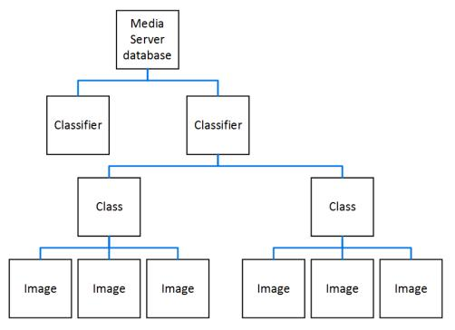
The "Media Server database" represents the Media Server datastore file or a database on an external database server. For information about how to set up this database, see Set up a Training Database, on page 43.
