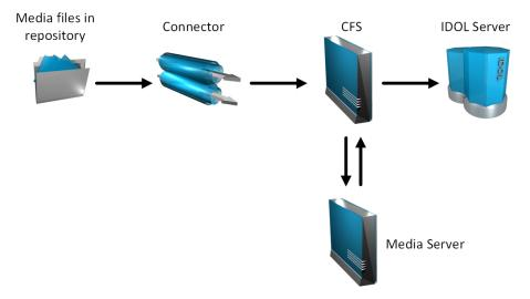
For example, a repository might contain video clips that you want to search or categorize. You could configure NiFi Ingest to send the video to Media Server and request analysis such as face detection, face recognition, object recognition, keyframe extraction and optical character recognition. Media Server returns information about the video content to NiFi Ingest, which might perform additional operations, such as Eduction, before indexing the information into an IDOL index.
