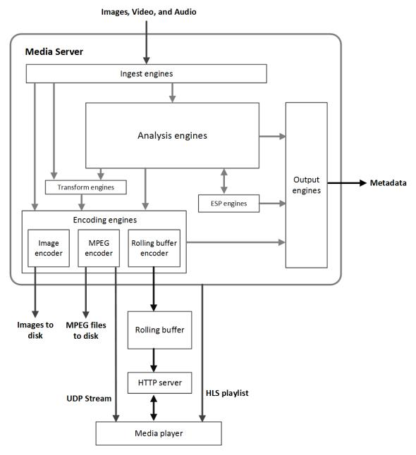
A Media Server *engine* performs a single function such as ingestion or analysis. There are several types of engine:
