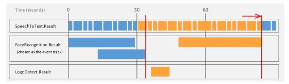
The end of the video is considered as an event, so in this case a final document is produced containing the final records in the speech-to-text result track:
