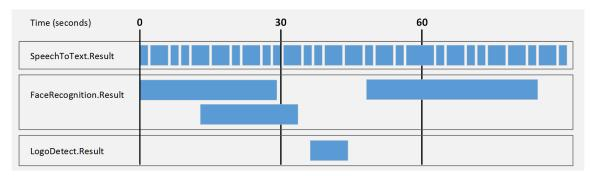
The first document contains the records related to the first interval (in this case, 30 seconds) of video content. Media Server does not output data at the 30-second point because a face recognition record has not ended (the face is still present in the video). Media Server can output data about the first interval as soon as this record ends:
