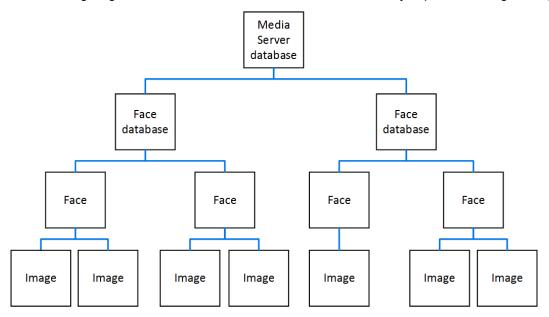
The "Media Server database" can represent either the internal Media Server database or a database on an external database server. For information on setting up this database, see Introduction, on page 43.
