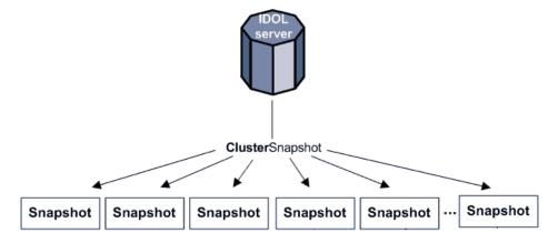
The ClusterSnapshot action allows you to take a snapshot of the data stored in the IDOL Content component data index. By default this includes data for the Content databases News and Archive. A snapshot represents the content of the data index at a particular time, and enables you to generate cluster information and spectrographs at a later point, even if the data index has changed. You can use a single snapshot to generate both cluster information and spectrograph data to save processing time.
