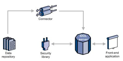
The connector retrieves information from your data repository and sends it to CFS so that it can be indexed it into IDOL server. The connector adds an encrypted ACL to each document. The ACL is in a custom format.
