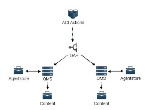
In a mirror mode configuration with multiple identical Content components, this architecture ensures that QMS is part of the load-balancing or failover that you use for your system.
