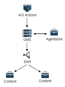
In a non-mirror mode configuration where your index is split over multiple Content components, this architecture reduces the number of additional components you need to configure. In a mirror mode
