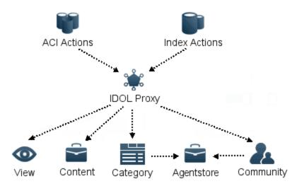
This setup is useful for training and testing, because it allows you to easily modify the configuration for the server, and you do not have to understand the whole IDOL architecture. However, for most production environments, the unified IDOL setup is too small and restrictive. For example, it has limited scalability and no failover, it is difficult to add additional Content components to increase the size of the index, and you cannot include QMS.
