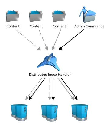
The DIH distributes the index data that it receives (represented by gray arrows in the diagram above) evenly across the connected IDOL Servers. For example, if the DIH connects to four IDOL servers, it
