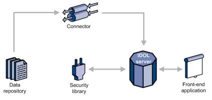
The connector retrieves information from your data repository and sends it to CFS so that it can be indexed it into IDOL server. The connector adds an encrypted ACL to each document. The ACL is in a custom format.
