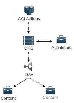
In a non-mirror mode configuration where your index is split over multiple Content components, this architecture reduces the number of additional components you need to configure. In a mirror
