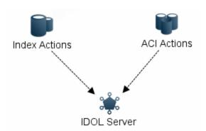
The unified setup uses the IDOL Proxy component. IDOL Proxy acts as a single point of contact for all your IDOL requests. It forwards all requests to the appropriate component. For example, it sends a Query action or indexing request to the Content component, and it sends a UserRead action to the Community component. IDOL Proxy also starts and stops the components in IDOL Server, and restarts components if they become inactive for any reason.
