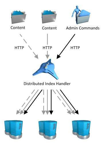
The DIH sends all the index data that it receives (represented by gray arrows in the diagram) to all the connected IDOL Servers. The IDOL Servers are exact copies of each other, and must all have the same configuration.
