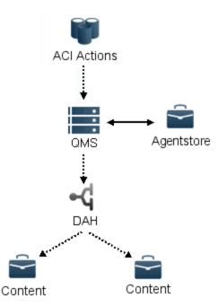
In a non-mirror mode configuration where your index is split over multiple Content components, this architecture reduces the number of additional components you need to configure. In a mirror mode configuration, you can use this architecture if you do not need to include load-balancing or failover for the QMS part of the system.
