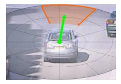
The length of the green arrow represents expected speed (pixels moved per second). The angle at which it is pointing indicates the expected direction of movement. The training utility also allows you to configure some variation in the expected speed and direction. In the example image, after one second has passed, the green dot at the center of the object can be expected to be located anywhere within the orange region.
