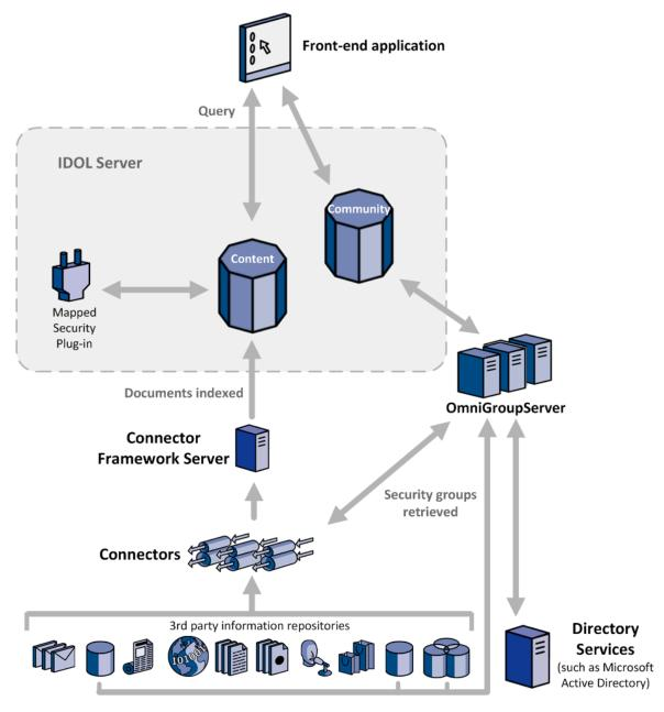
Connectors extract information from third party repositories so that the information can be indexed into IDOL Server. The connector adds an Access Control List (ACL) to a metadata field in each document. The ACL describes which users and groups are permitted to view the document. CFS indexes the document into IDOL Server.
