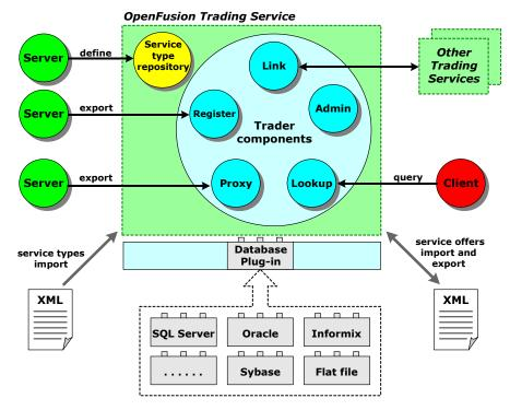
Figure 2 Structure of the Trading Service
