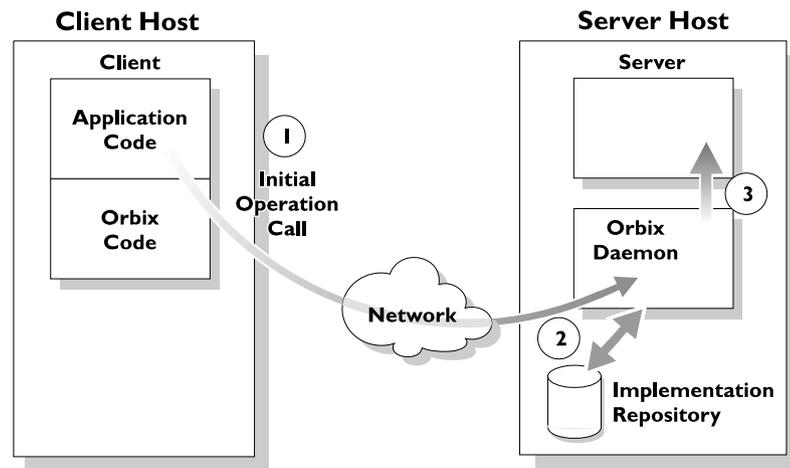
Figure 2: Automatic Launch of an Orbix Server Process
