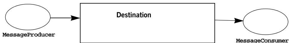
Figure 7: Simple JMS system
