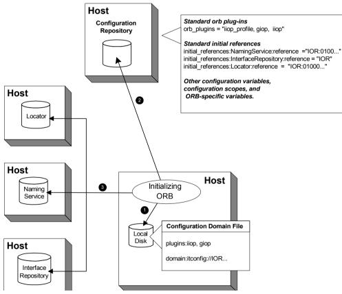
Figure 11: How an Orbix Application Obtains its Configurations
