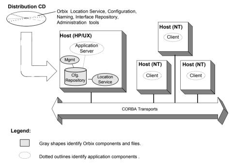
Figure 10: Orbix Environment with Centralized Configuration
