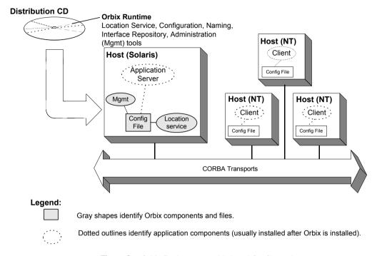
Figure 9: Orbix Environment with Local Configuration
