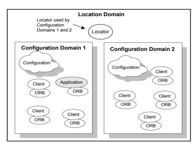
Figure 5: Multiple Configuration Domains
