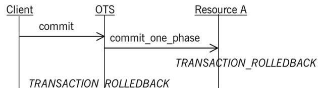
**Figure 11:** The 1PC protocol resulting in a rollback.
