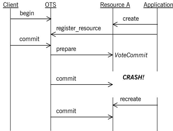
**Figure 13:** Recovery after the failure of a resource object
