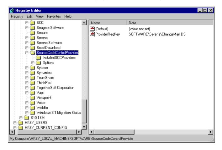
The following figure shows is the Windows registry editor after the SourceBridge installation. The ProviderRegKey points to SBM. The prior setting of ProviderRegKey is saved in SerenaCopyofOriginalProviderRegKey.
