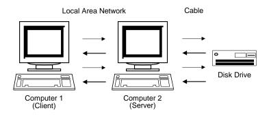
In <u>Figure 21</u>, Computer 2 acts as a conduit, called a server, through which the requests of Computer 1, called a client, are routed. (The server routes requests for more than one client computer, which is an advantage of local area networks.) A more effective way to route requests, however, is shown in <u>Figure 22</u>.
