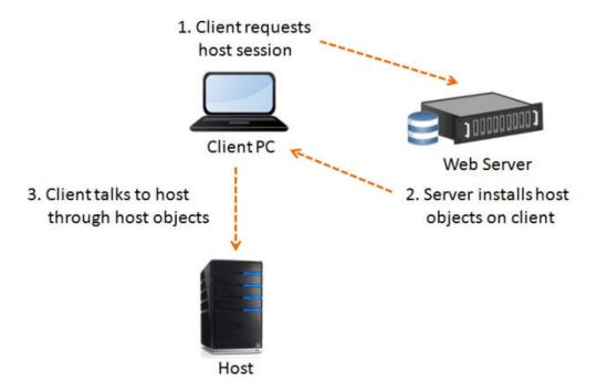
The ActiveX objects and JavaBeans are downloaded to the client the first time a user opens a session. When you install updates on the server, they are downloaded automatically to the client the next time a user opens a session. This architecture enables the client to communicate directly with the host, as shown in the figure above.
