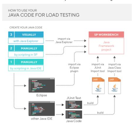
Depending on how you import Java code to the Workbench, Silk Performer creates different sets of files within the Java Framework project. This results in different call sequences. The diagram below shows three types of call sequences:
