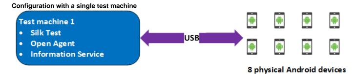
Using a single test machine directly connected to the Android devices through USB, we tested up to 8 physical Android devices in parallel.
