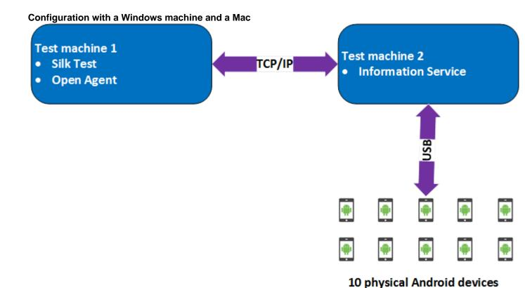
Here we are using two test machines, a Windows machine with Silk4NET installed and a Mac, which is configured as a remote location for the first machine and has the Silk Test Information Service installed. Using such a configuration, we tested up to 10 physical Android devices in parallel.
