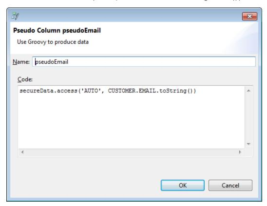
For similar identification of the de-identified (encrypted) data, you can use protect method available in secureData object to encrypt (or de-identify) the data in DAC. The following methods are available for the same:
