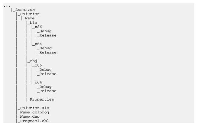
If you select the Create Directory for Solution option when creating a solution, the structure is slightly different.
